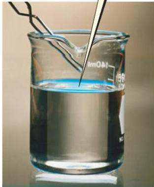
Seed crystal of sodium acetate added to supersaturated solution
