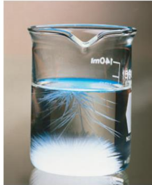
Excess sodium acetate crystallizes from solution
