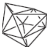
9-coord tri-capped trigonal prism
